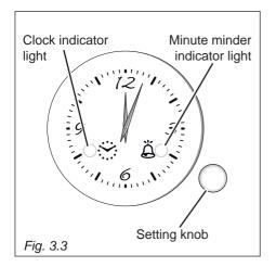
ATTENTION - MOST IMPORTANT: This is only an alarm that DOES NOT switch off the oven or grill. REMEMBER TO TURN OFF THE OVEN OR GRILL MANUALLY.
